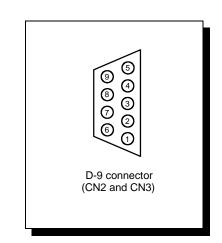
Figure 23 --- DSC-200/300 output connectors
