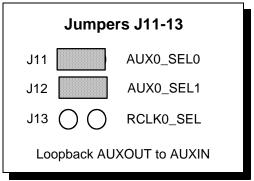
Figure 19 --- AUXIN/AUXOUT loopback
