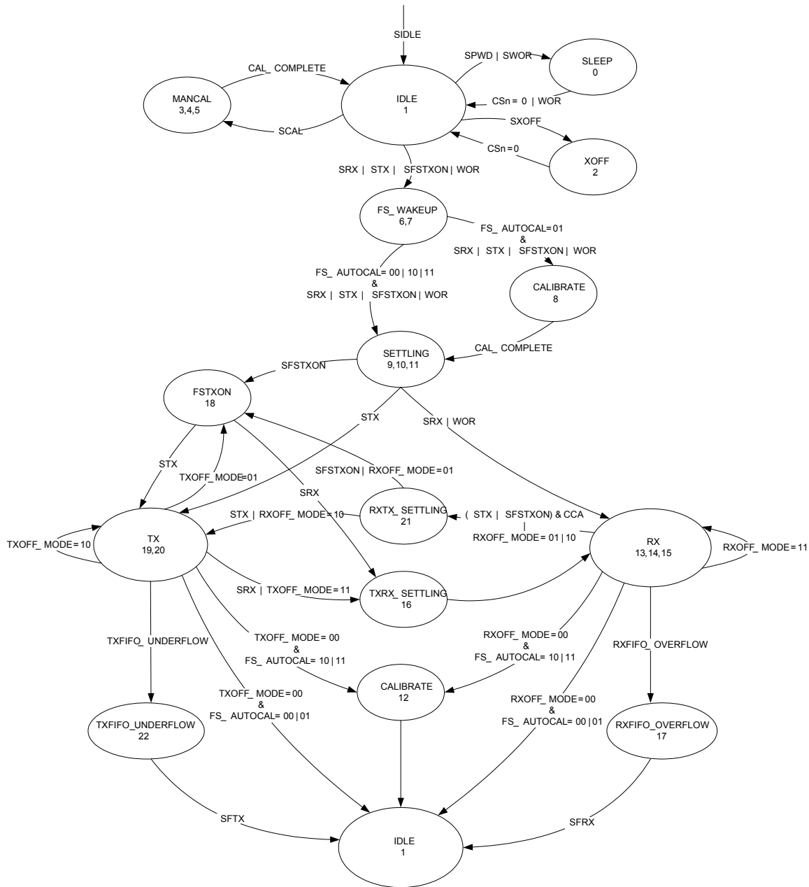
Figure 15: Complete Radio Control State Diagram
